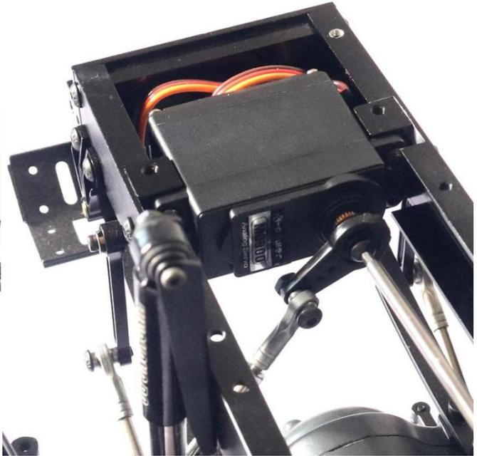
Install the variable speed steering gear (the steering gear needs to be purchased separately)
