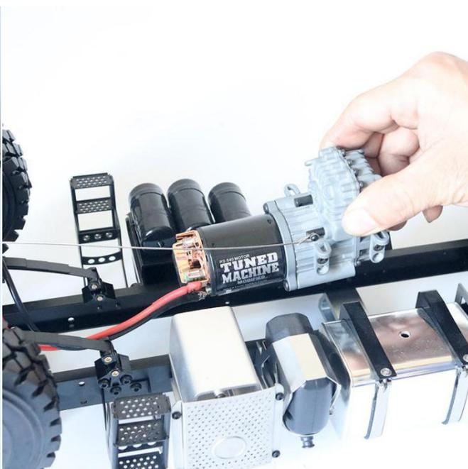
Put on the cable, fasten the cable screw with proper force, and ensure the sheath fastening passes through smoothly
